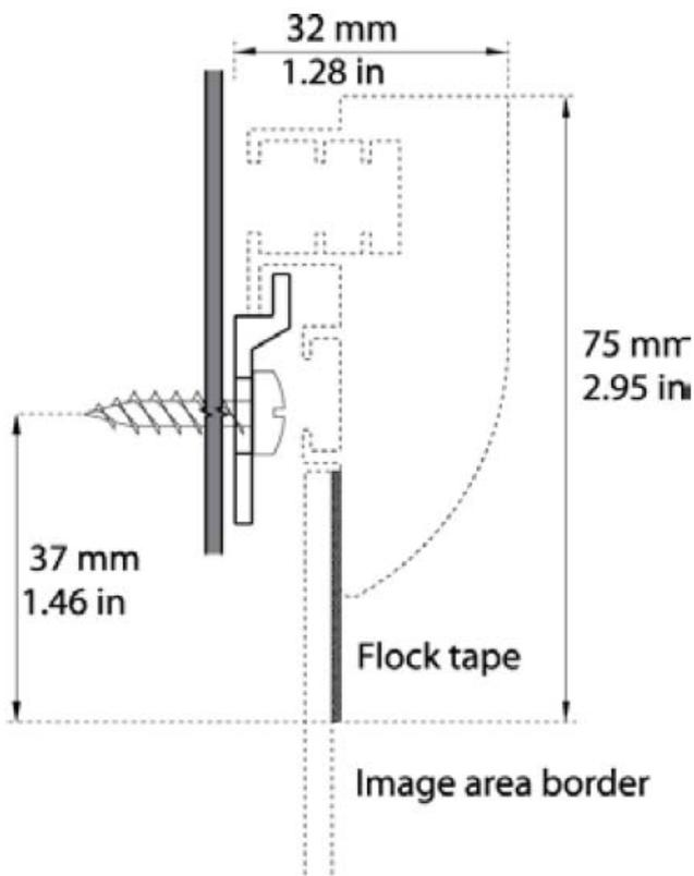
Place the screws 37 mm (1.46 in) above the desired image area's top border. Position the brackets approx. 150 mm (5.91 in) from the outer edge of the frame.
