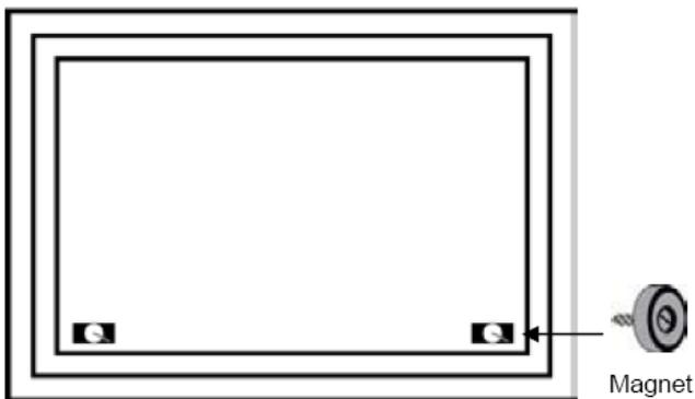
Put a screw into each of the magnets and attach them to the centre of each of the two backplates by using magnetic force (screw tips should face away from the screen).
