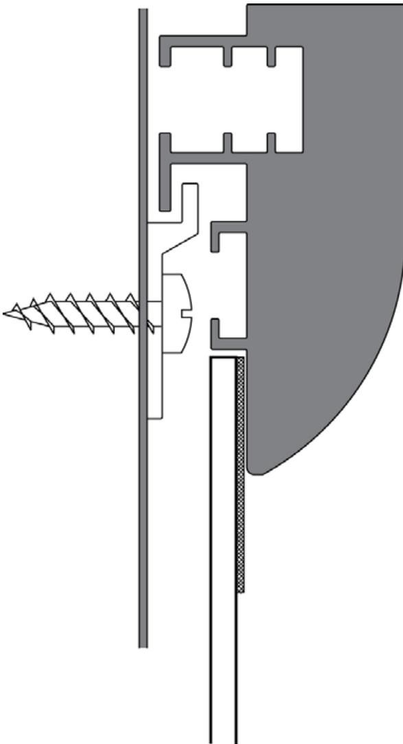
Lift the screen up against the wall, slightly higher than the brackets. Then let it slide down on the brackets until they are firmly in position. Only tilt the screen slightly during this operation, as it can loosen the brackets.
