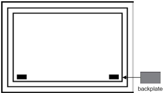
The backplates ensure that the screen is fixed firmly to the wall. Remove the covering from the tape and glue the two plates into position in each lower corner of the screen's back side. If the wall is uneven, you may have to find a more suitable position than the lower corners.
